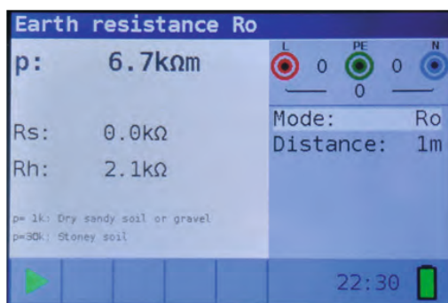
Figure 4 41: Example of specific earth resistance measurement results
