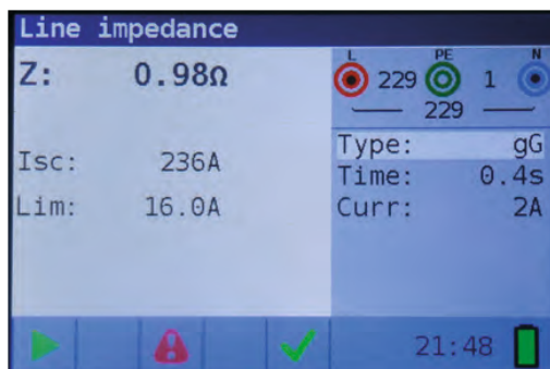
Figure 4 28: Example of line impedance measurement results
