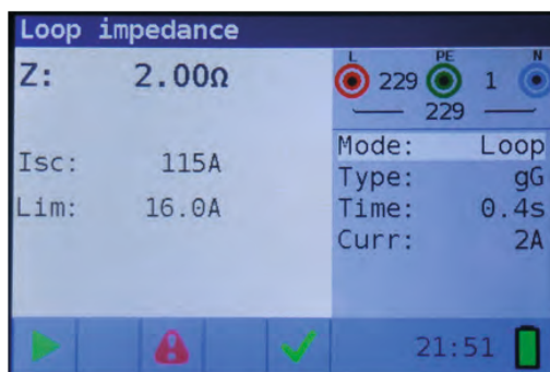
Figure 4 23: Example of loop impedance measurement results
