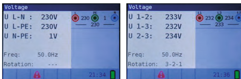
Figure 4 34: Examples of voltage and frequency measurements
